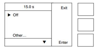
The top line displays the current setting. The values shown are for the CP1 (the values for the CP2 are shown in brackets). Use the keys to select one of the five options available. The **Other** menu allows any time between 1 and 59 seconds for the CP1. The time is set in 1 second increments.
