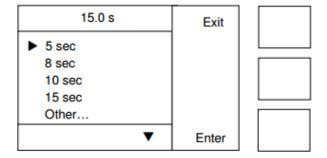
Use the keys to select one of the five options available. The **Other** menu allows any time between 5 and 59 seconds to be set (in 1 second increments). This time should always be at least 15 seconds.
