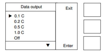
Note that the temperature (shown at the top-left of the display) will flash when the plate temperature is more than the ready band temperature-difference away from the set temperature.
