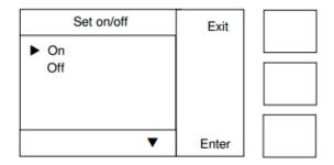
The following screen appears once the **Minimum** menu has been selected. Once enabled, the minimum value during a run will be displayed on the result screen.
