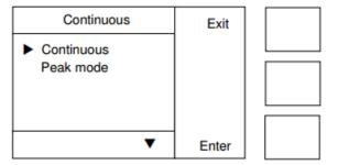
The top line displays the current setting. Select **Continuous** mode (default) to report the viscosity value at the end of the run time or select **Peak mode** to report the maximum (peak) viscosity value (at the end of the run time).
