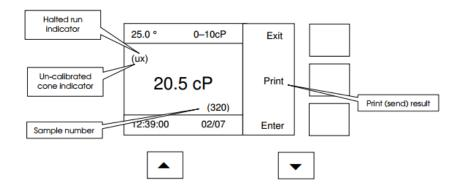
The **Print** key becomes visible once a result has been taken (manual mode only). Print (after result) is always enabled when the instrument is in automatic mode. Results are always printed in cP (mPas).
