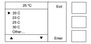
Use the keys to select one of the four pre-set values. Alternatively, the temperature may be set to any value between 5°C and 65°C in 0.1°C increments when the **Other** menu is selected (see the next section). Select **Enter** once the required temperature has been chosen. The instrument will quickly change to the new set-point. Once the new set-point has been reached, a delay of 20 seconds is used to allow the plate surface-temperature to reach the precise set point.
