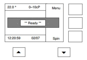
The bottom right-hand key indicates that the cone can be rotated to aid cleaning (since the handle is up at this point).
