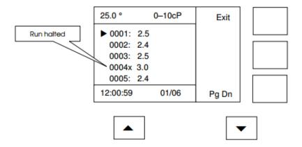
In this case, the temperature, cone, date and time refer to the highlighted line, so as the select arrow is moved down, these values change showing the results recorded for that run. The 'x' on the fourth line indicates that the run was halted prematurely. When limits are enabled, any result outside the pre-set limit values will be shown in reverse video.
