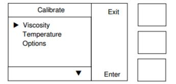
Choose either viscosity (torque measurement) or plate temperature calibration. The options section allows the calibration time to be altered from the default 20 seconds value.
